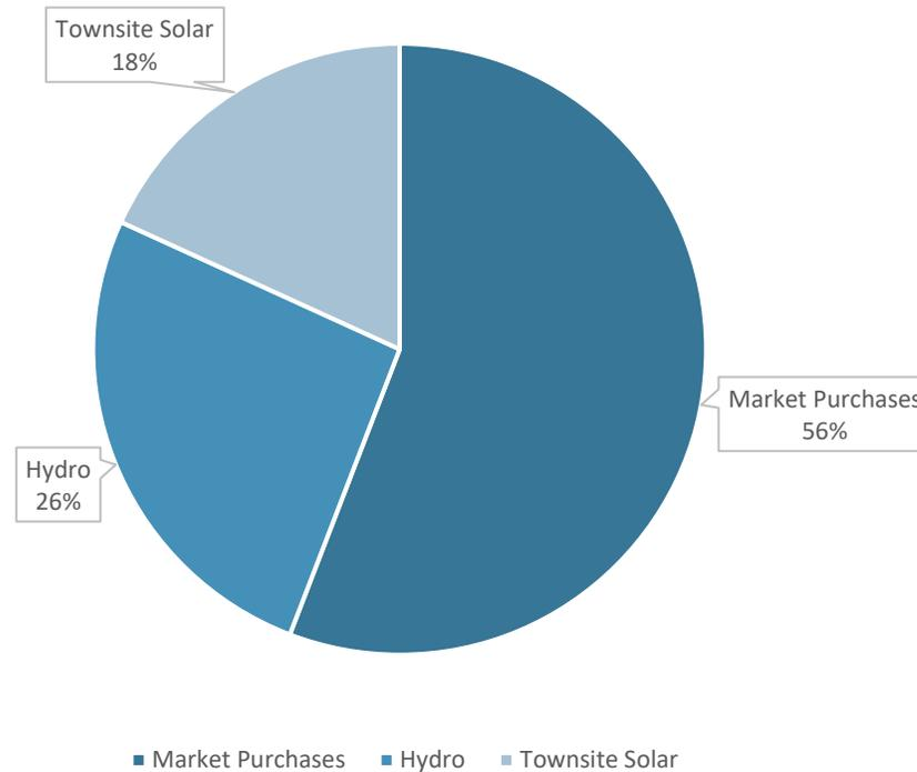
BOULDER CITY'S ENERGY DISTRIBUTION FOR FEBRUARY 2023 DERIVED FROM HYDRO, TOWNSITE SOLAR AND MARKET PURCHASES. MARKET PURCHASES MADE UP MOST OF THE ENERGY DISTRIBUTION WITH 10,326 MWH. THE CITY RECEIVED 4,809 MWH OF HYDRO, AND 3,360 MWH FROM TOWNSITE SOLAR.
